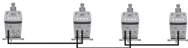
Fig. 19: Synchronization of several dosing pumps by means of stroke feedback and pulse control
